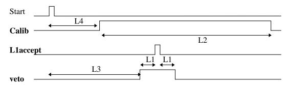
At the output of the **PDC** module all these signals are synchronized to the **PDC** clock. At the output of the **Fan-out** modules, **L1accept** will still be synchronized to **CLK**, but **Calib**, which is not delayed, will no longer be synchronized.
