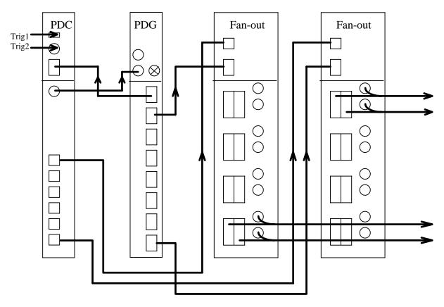
The system outputs are designed to be compatible with the inputs needed by the frontend cards: the FEB, the calibration board and the mini-ROD. Each output is conform to the specifications for the fast signals defined in the Nevis workshop; it is composed of a bundle of the following five signals:
