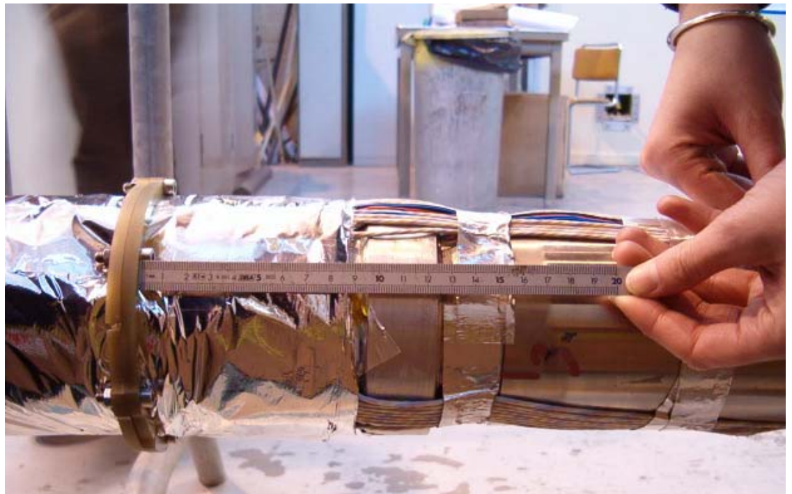
Figure 14: The warm tube. The 6-mm thick ring of the bi-metal junction, located in 11 cm from the spacer, is seen. A bunch of wires (PT100 probe signals, heater power) make the narrowest gap between the warm and the cold tube. The cold sensors 61 and 69 were located in about 5 cm from the spacer.
